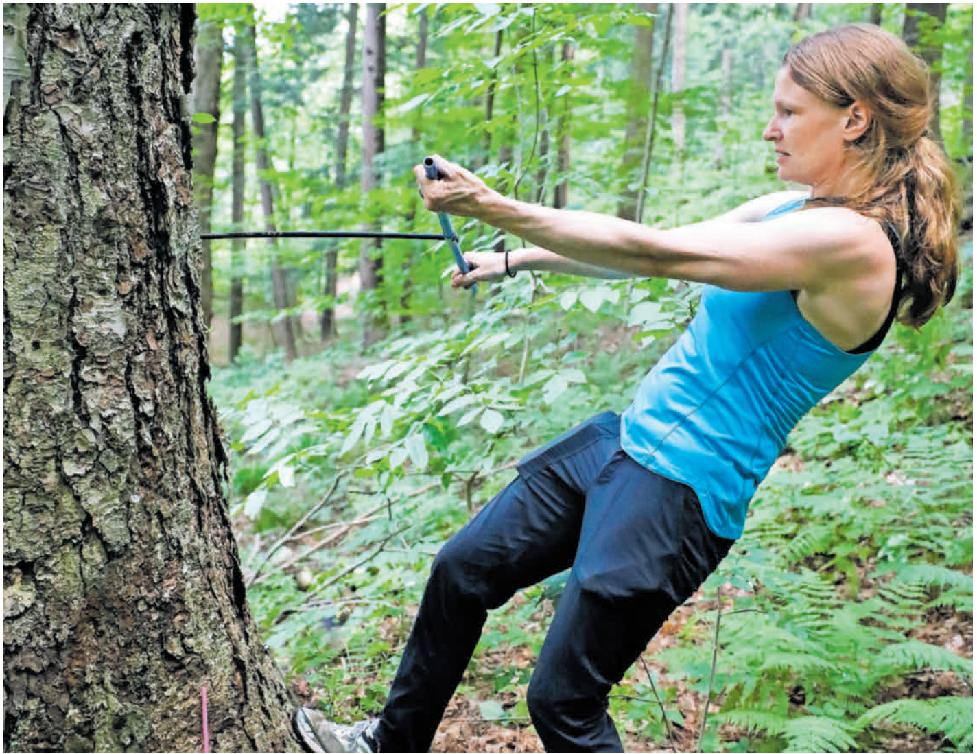
Research assistant Laura Smith uses an increment borer to get a core sample from a tree. Hardwood trees are often too dense for power tools to penetrate all the way to the center.
