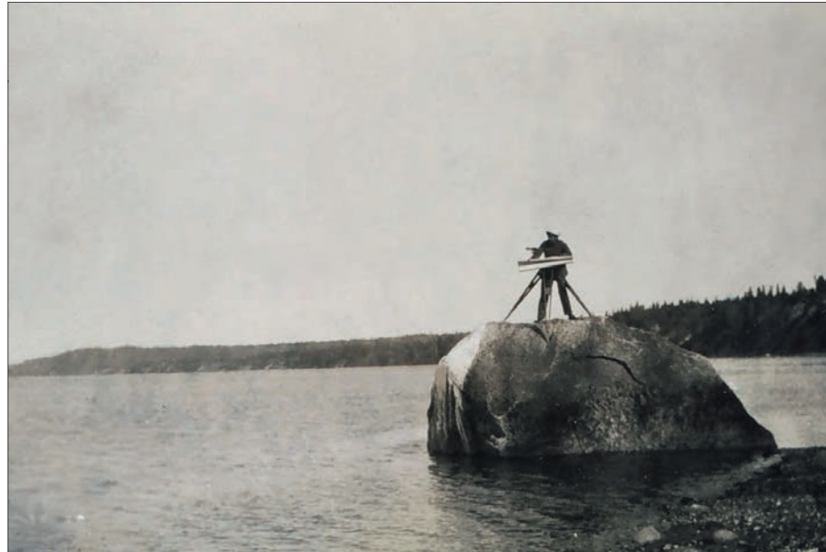
Figure 5. Coast Survey plane table mapping. The surveyor is using the plane table on an offshore rock in Cook Inlet, Alaska, circa 1910. The alidade can be seen on top of the surface of the plane table (U.S. Coast and Geodetic Survey c. 1910).
