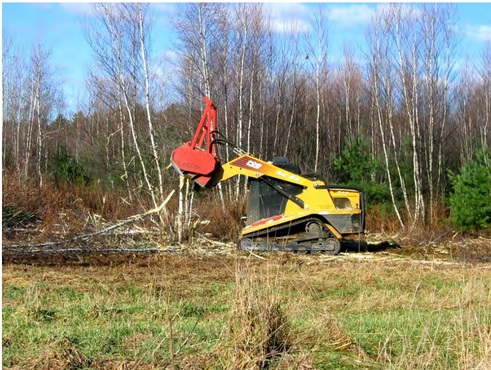
An ASV with a fecon head mulches birch in an abandoned agricultural field
